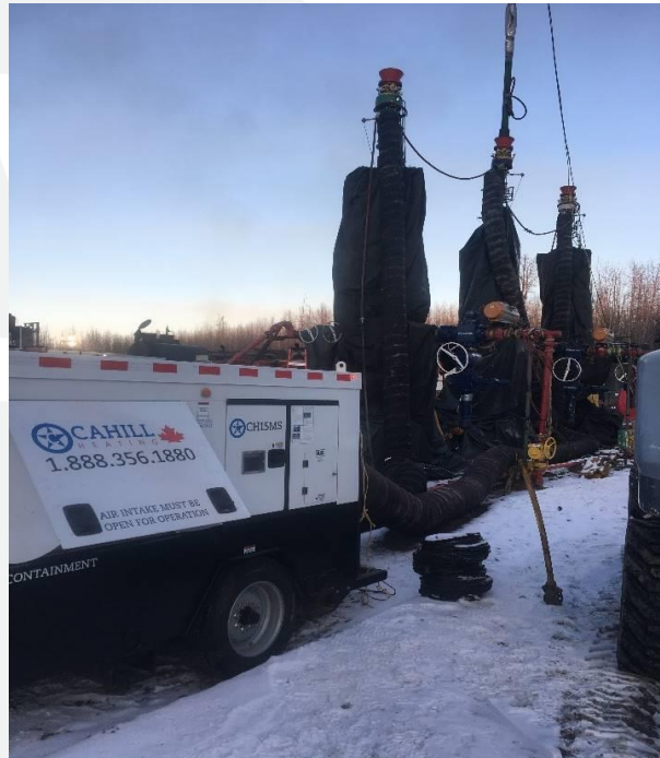
A CH15MS heater heating multiple BOPs simultaneously using split ducting on an oilfield
